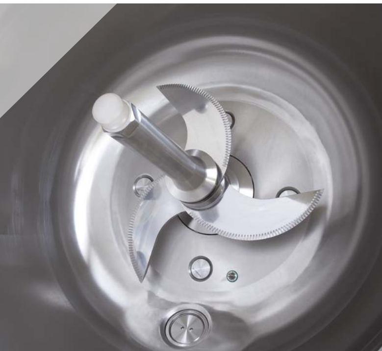
Steam injection nozzles and knives
